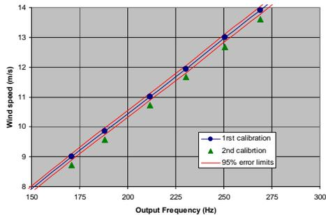
Figure 6. Recalibration results – unit with bearing damage, 15 months of operation on site
