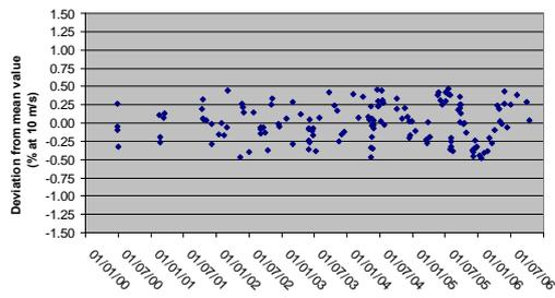
Figure 3. Results from Reference anemometer calibrations.
