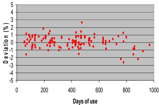
Figure 7. Deviation at 10m/sec for recalibrated units, as a function of usage time (Vector A100K, 137 cases)
