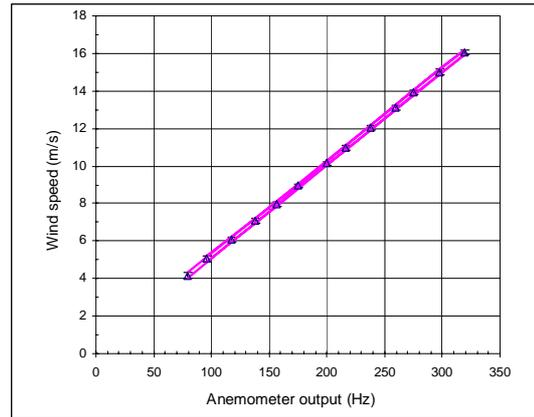
Figure 4 Response characteristics of a VECTOR A100K cup anemometer with calibration error limits (typical error 95%)
