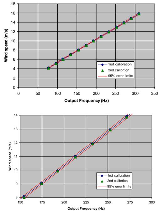
Figure 5. Recalibration results – undamaged unit, 15 months of operation on site
