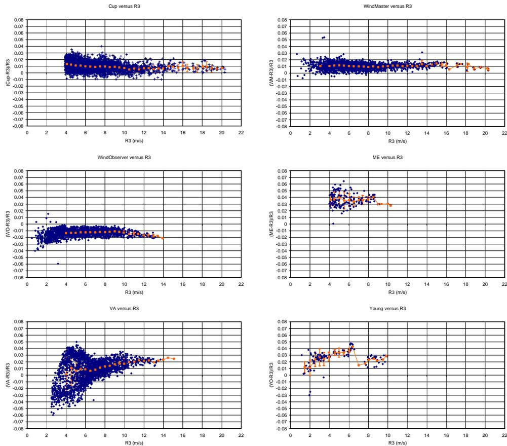
Figure 4-11 Relative difference of cup and test sonic anemometers to Solent R3A sonic measured on sonic field comparison test rig
