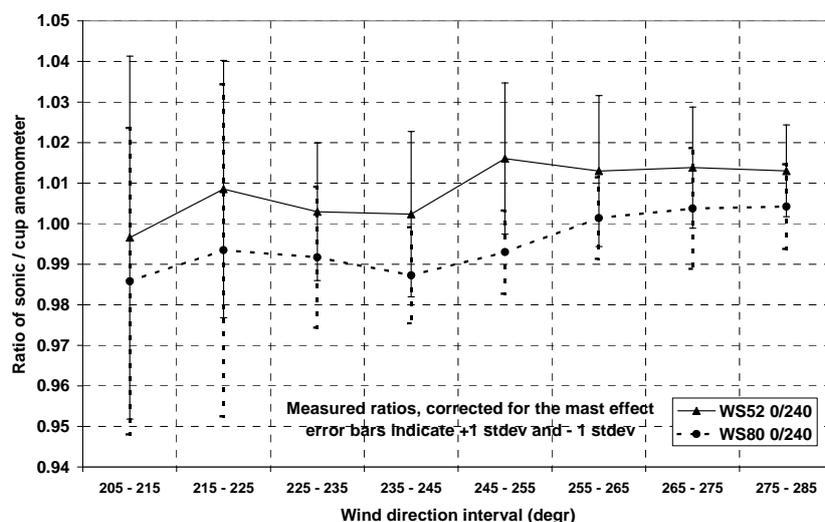
Figure 4-9 Ratios (corrected for mast and boom effects) between the Gill Wind Master sonic anemometer ( $0^\circ$  boom direction) and the cup anemometer ( $240^\circ$  boom direction) at 52m and at 80m, including the  $+1\sigma$  and  $-1\sigma$  error bars.
