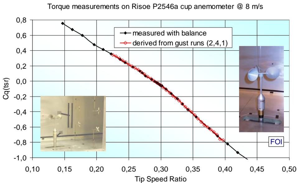
Figure 4-3 The graph shows a comparison of  $C_q$  in vertical position for the Risø P2546 cup anemometer measured with the static and the dynamic torque measurement methods. Speed ratio from dynamic measurement has been offset by  $-0.006$  and  $C_q$  scaled up by 7% (rotation around  $C_q=0$ )
