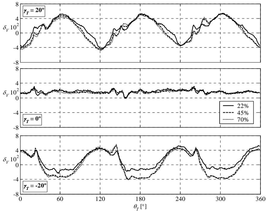
Figure 4-7 Results for the percentage deviation in the measurement of the total wind speed as function of the true wind direction relative to the sensor for three different inclination angles. Percentages indicating wind speed (22% $\approx$ 4.34 m/s; 45% $\approx$ 9.89 m/s and 70% $\approx$ 15.99 m/s). Gill Wind Master at IDR wind tunnel
